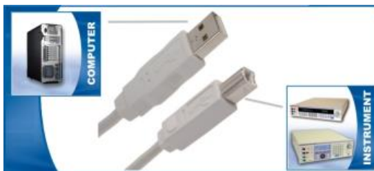
Figure 5 - USB Cable Connection from PC to Instrument
