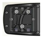
Install the three batteries by sliding them into the bottom of the battery slots, making sure the polarity markings on the batteries align with the markings shown in the battery compartment.
