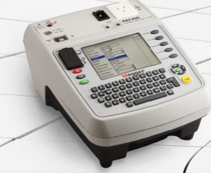
Operators of electric tools and other electrical equipment must be protected from potentially dangerous flaws in workmanship or wear and tear. The PAT450 is designed to test portable electrical equipment for safe operation.
