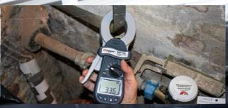
Designed with flat core ends, they prevent dirt build up, ensuring measurement integrity and improved reliability over products with interlocking teeth. Other enhancements over current generation products include improved accuracy and up to 300% increase in battery life. In electrically noisy environments the built-in filter function offers increased noise immunity.
