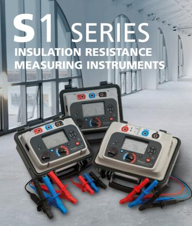
Megger's S1-Series of insulation resistance testers consists of 5 kV, 10 kV and 15 kV models called S1-568, S1-1068 and S1-1568. These class-leading instruments are targeted at power utilities and service companies working in generation, transmission and distribution markets. Class leading charge current, noise rejection and software filters make the S1-Series Megger's most advanced DC insulation resistance testers to date.
