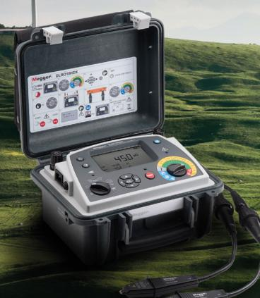
Augmenting Megger's DLRO10 and 10X range, the DLRO10HDX combines ultimate simplicity of operation with a rugged IP65 case designed for stable ground and bench operation and provides memory storage.
