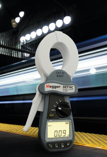
The DET14C and DET24C represent a new generation of earth/ground clamp-on resistance testers. These instruments induce a test current into earth systems and measure ground resistance in multi ground installations without needing to disconnect the ground. They offer market leading access, advanced features, simple operation and CAT IV 600 V safety protection.
