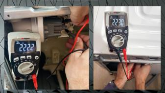
The AVO215 true RMS multimeter is a rugged compact instrument for demanding environments. It measures true RMS voltage up to 600 V and current to 10 A with 4000 count resolution. As well as resistance, continuity, frequency, and capacitance for quick verifications, it meets CAT III 600 V AC/DC safety and contains a built-in flashlight, making it ideal for wide range of applications.
